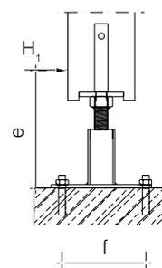
$$R_{\text{axial,Bolzen}} = \frac{H \times e}{f}$$
