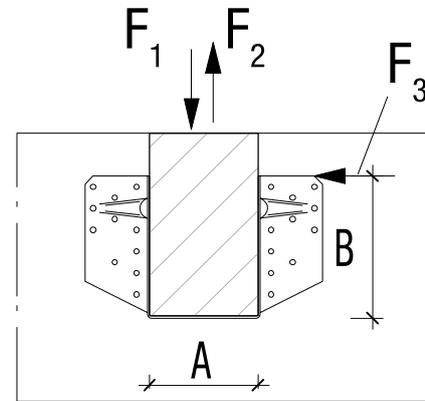
$$\text{Es gilt: } \left( \frac{F_{1/2,d}}{R_{1/2,d}} \right)^2 + \left( \frac{F_{3,d}}{R_{3,d}} \right)^2 \leq 1,0$$
