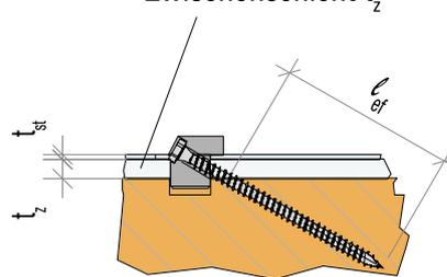
$$l_{ef} = l - (t_{st} + t_z) \times 2$$
